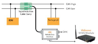
The VDI module is then connected to the WIMS data logger that runs periodic collections of this data via its RS232 port and then reports back to the Vidiwave Cloud management platform (Vidi-Cloud).
